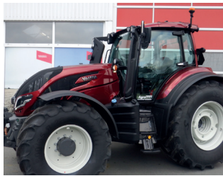
NY Valtra T255 Versu 250 hk. - Affj. foraksel - Affj. kabine - Frontlift - 600/65x28 - 650/75x38 - Submeter GPS - LED lys
