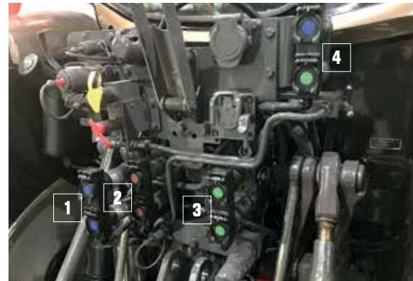
Location of the rear valve quick couplers.
